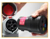
The markings and the colors of the banana female connections show me where to connect to the phases, the neutral, the protective earth, and the pilot.
